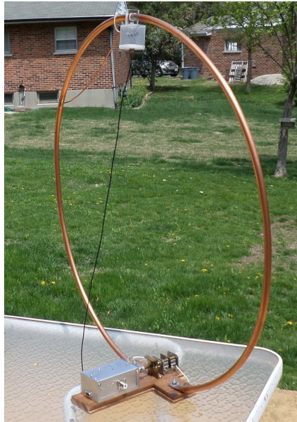
Figure 4. Loop antenna and stepper motor/swr indicator assembly.
