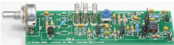
a stand-alone QRPp transmitter with 250mW of output power.
