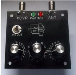
Designed by David Cripe, NM0S (4sQRP #12), this is a classic T-Match tuner with a wrinkle – the SWR indicator employs 2 LEDs instead of the normal single LED. The green LED indicates forward power, while the red indicates reflected power. The board features “Pittsburg” construction techniques developed by Joe Porter, W0MQY (4sQRP #103), making for a very easy build!
