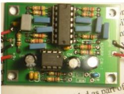
Designed by David Cripe, NM0S (4sQRP #12), this is a small, high-performance audio filter. This is a flexible design that can be used stand-alone, or integrated into an existing receiver. It features a 200 cycle bandwidth with no ringing.
