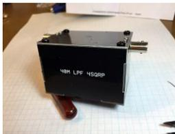
Designed by David Cripe, NM0S (4sQRP #12), this design uses the “spiral coils” made popular in the retired NS-40 transmitter. Also included is the PC-Board case, which is another hallmark of David’s designs. The filter is available in either an 80 or 40 meter version. This was the build session kit for Ozarkcon 2015, so it’s a very easy build!
