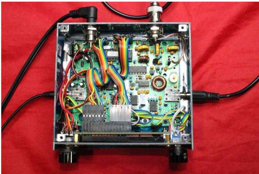
The board is 10 by 8 centimeters and the LCD display is a standard sized 16 X 2 character display with a blue back light. The antenna connector is on the right side and protrudes from the board. The key jack is also on the right and protrudes slightly with the earphone jack on the left side
