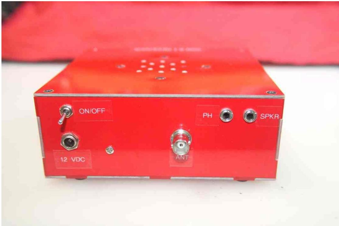
About then, our fantastic kit designers came up with the AA0ZZ PC material enclosures and I obtained one of each size that was available at the time. The PC board for the SSB 6.1 was a bit too large for the small (Little Blue Box) enclosure, so I did a quick layout to see if it would go into the medium (Little Red Box) enclosure and fortunately there was enough room to put everything in there.
