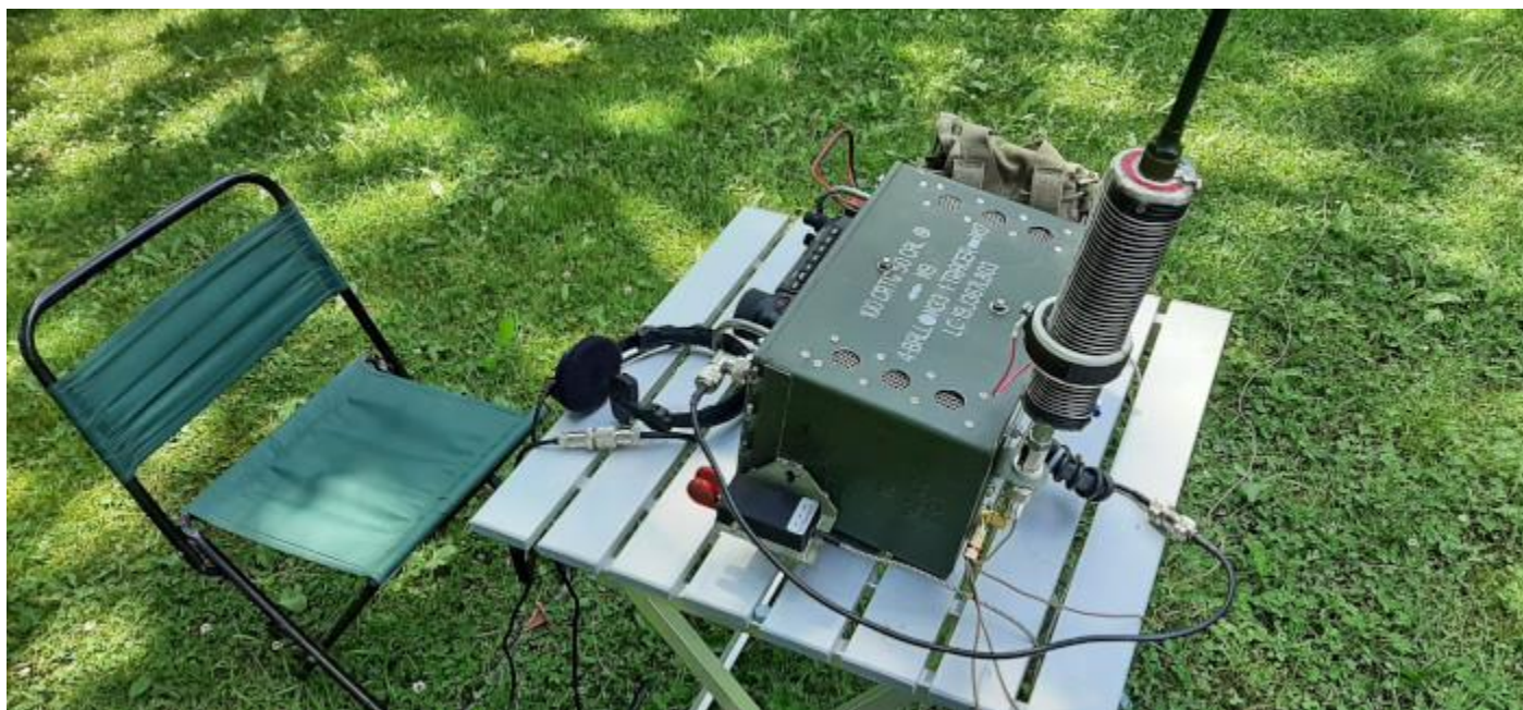
VA3KOT's trail-hardened FT-891 rig with ham-made adjustable loading coil and 9.5ft top-hat loaded whip
