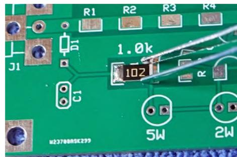
Next, simply apply solder to the other pad using just enough solder to securely mount that side of the part. You can “touch up” the solder on the first pad if needed to remove excess solder or add solder.
