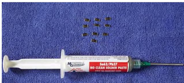
Put a dab of solder paste on each pad and then use tweezers to place the parts on the pads. The paste will hold them relatively stable. Don't be concerned if a little paste oozes out and looks a bit sloppy.
