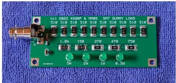
Using either method, start the SMT installation with the five values on the lower row. The 1.0K ohms resistor is marked "102", 150 ohms is marked "151", 270 ohms is marked "271", 470 ohms is marked "471" and 750 ohms is marked "751".
