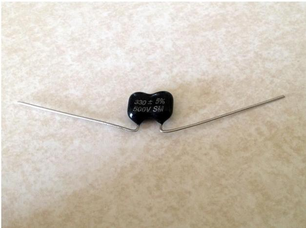
Bend capacitor leads thusly for easy soldering and trimming. This is the "Pittsburg Bend" for Silver Mica caps.
