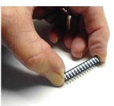
you've installed the IC, ensure that all leads are seated in the socket.
