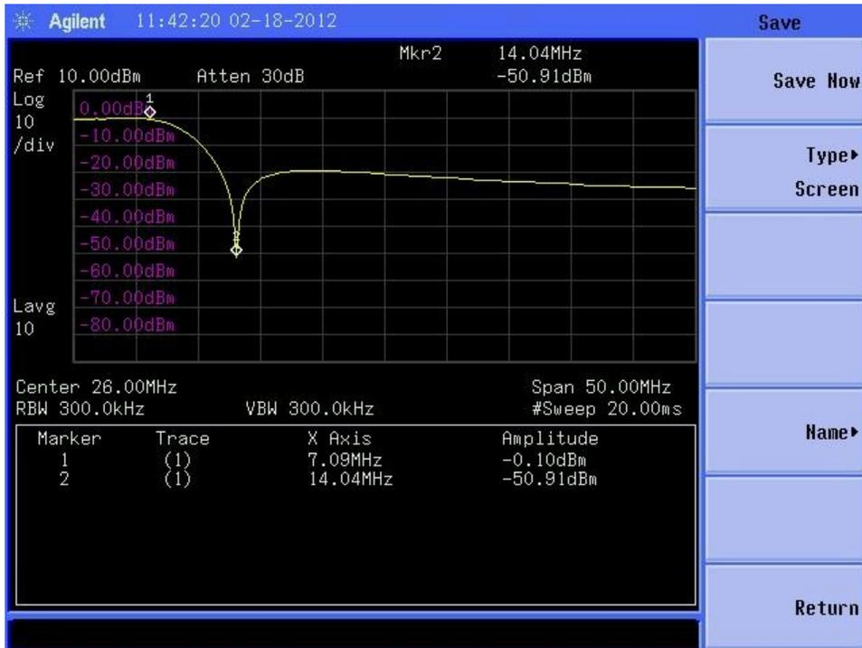
The 50 dB notch in the response is positioned where the 2<sup>nd</sup> harmonic will fall. Also notice, the loss through this filter is very small, on the order of 0.1 dB, so will not waste much power; a few milliwatts at most.
