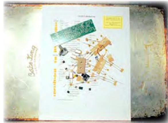
4SQR Group specs the SAVXO with 250 mW of RF power, and suggests it may be used as a standalone QRPP transmitter by adding a low-pass filter. Jury-rigging the SAVXO into the NorCal Power Meter (*K9YA Telegraph*, November 2008) followed by a dummy load and adjusting onboard trimmer TR1, the measured output ranged between 0 and .3 watt.
