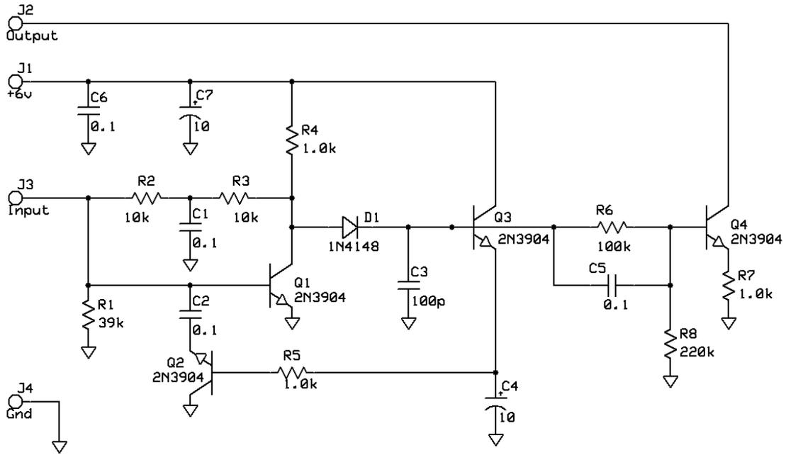
Figure 1: AM Detector Circuit with AGC.
