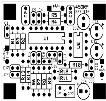
Figure 2: Component Placement
