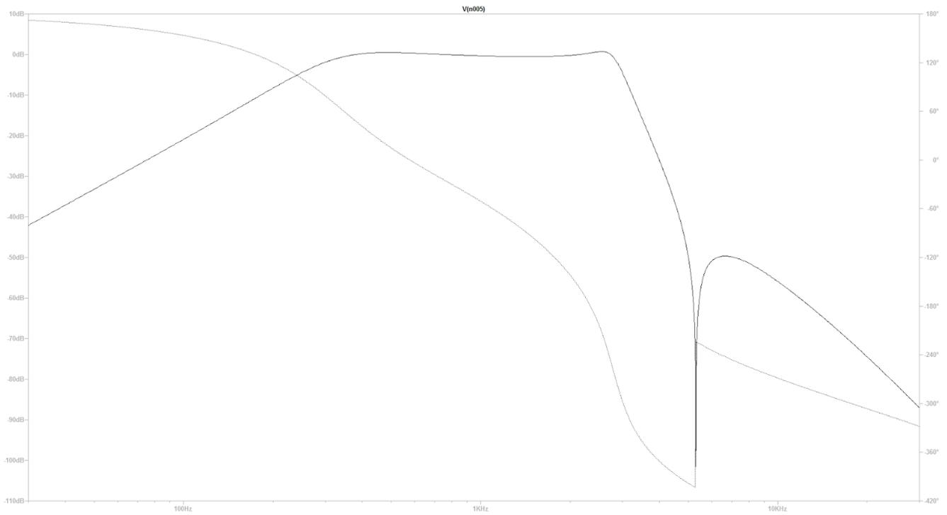
Figure 1: Frequency Response of SSB-Mite Filter
